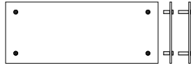
kit 104 V (kit B 30 / kit B 50) w 750 x h 300 x d 8mm w 29,53 x h 11,8 x d 0,31"
